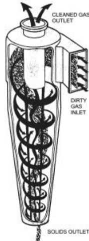
Figure 11 Diagram of a typical cyclone
